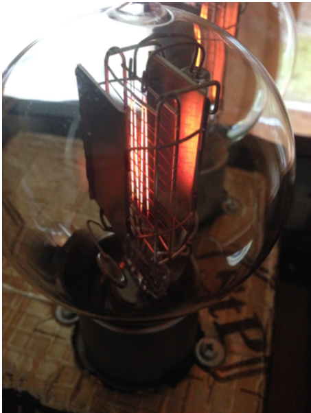
Above: the WE 101D replica triode (designed 100 years ago in 1914. )
