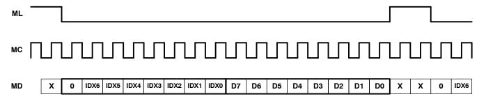
Figure 24. Register Write Operation
