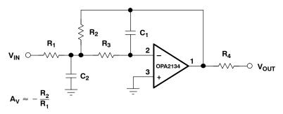
Figure 29. Dual-Supply Filter Circuit
