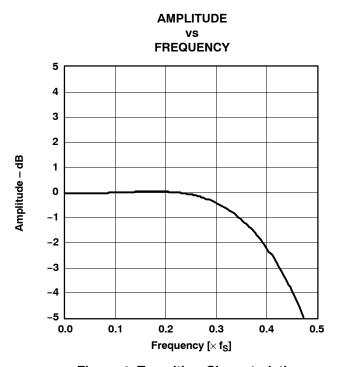
Figure 4. Transition Characteristics, Slow Rolloff
