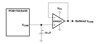
(b) Using a Voltage Follower to Buffer  $V_{\text{COM}}$  When Biasing Multiple Nodes
