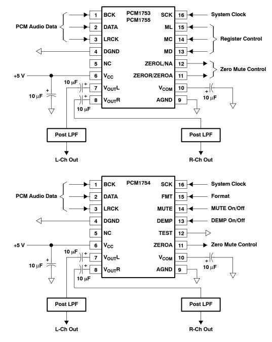
Figure 28. Basic Connection Diagram
