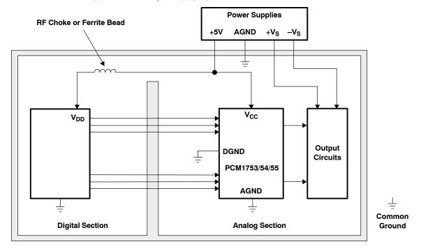
Figure 31. Single-Supply PCB Layout
