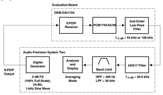
Figure 36. Test Setup for THD+N Measurement
