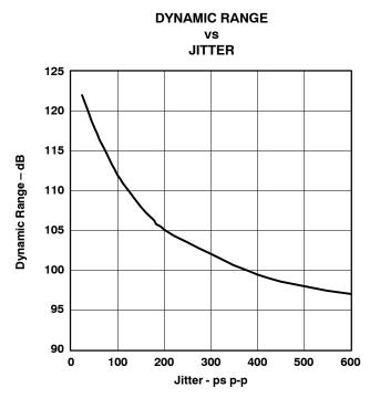
Figure 35. Jitter Dependence (× 64 Oversampling)
