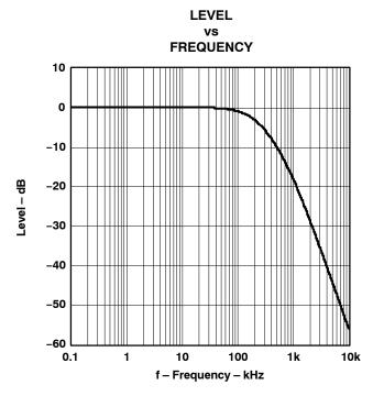
Figure 26. Output Filter Frequency Response
