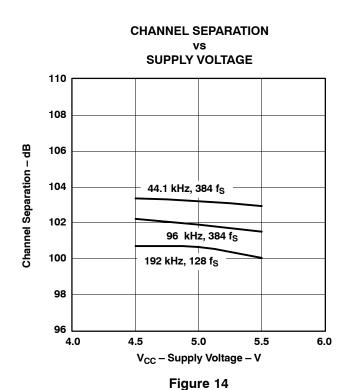
All specifications at  $T_A = 25$  °C,  $V_{CC} = 5$  V,  $f_S = 44.1$  kHz, system clock = 384  $f_{S_1}$  and 24-bit data, unless otherwise noted
