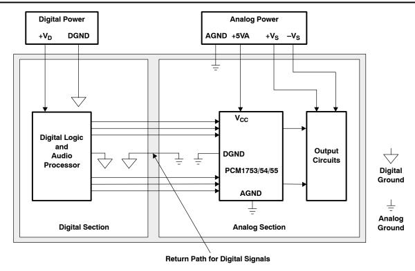
Figure 30. Recommended PCB Layout
