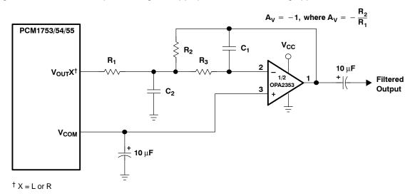
(a) Using V<sub>COM</sub> to Bias a Single-Supply Filter Stage
