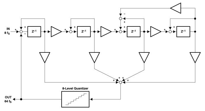
Figure 32. Eight-Level Delta-Sigma Modulator
