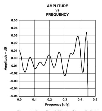
Figure 2. Pass-Band Ripple, Sharp Rolloff
